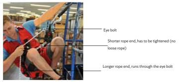
Using the eye bolts, you can control the descent speed or stop the descent. The longer, unloaded rope end runs through the eye bolts. If you hold on to the longer rope end, you can throttle the descent speed or stop the descent. If you don't use the eye bolts, the descent speed will be regulated automatically by two fly wheel brakes (speed ca. o.8m/sec)
